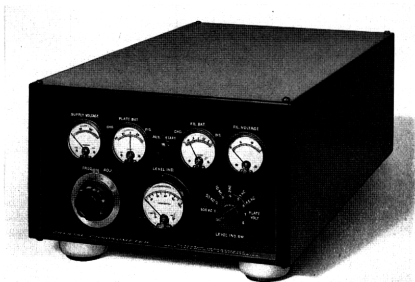
Fig. 33—Crystal chronometer for geophysical studies, consisting of 100 KC. GT-cut crystal, bridge oscillator, and frequency converters to derive precision 500-Cycle output to operate timing devices.
